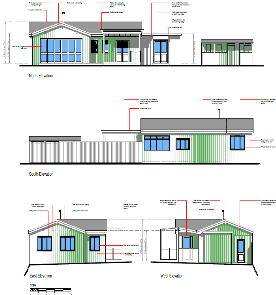
Fig 1: Initially Proposed Elevational Drawings with Proposed Extensions to the Existing Building (not to scale).
